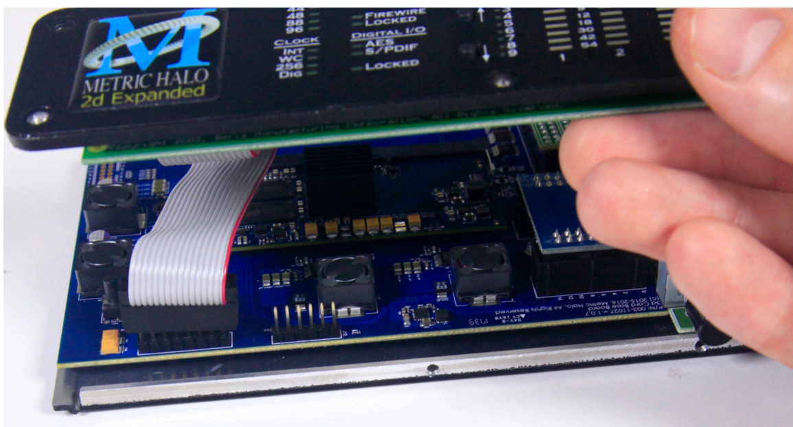
Figure 1.26: Reattach Meter Board
