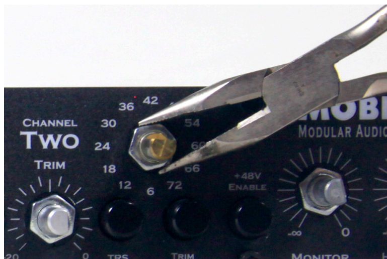
Figure 1.15: Remove Front Panel Hex Nuts
