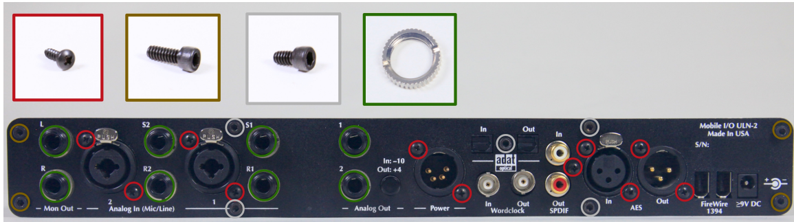
Figure 1.20: Screws and Nuts to Remove from Back Panel
