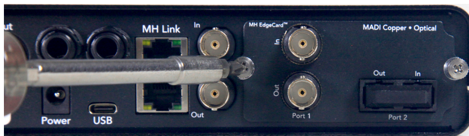
Figure 16.18: EdgeCard Installed Available for Routing in MIOConsole3d
