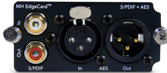
Figure 16.5: MH EdgeCard: SPDIF • AES
