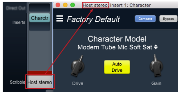
Figure 3.15: Scribble Strip name to Mixer strip Insert header
