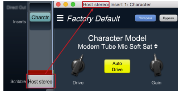
Figure 4.15: Scribble Strip name to Mixer strip Insert header
