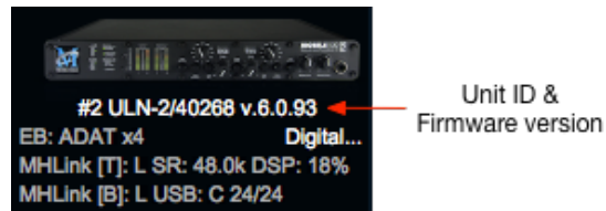
Figure 10.79: Unit ID and Firmware version
