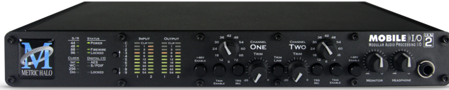
Figure 7.2: Mobile I/O Unit
