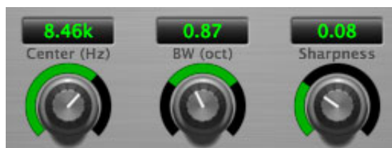
Figure 13.167: Ess Band Filter Controls
