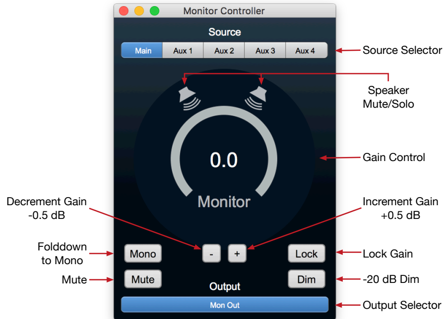
Figure 11.1: Monitor Controller controls
