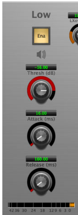
Figure 13.157: Expander (Low Frequency Shown)
