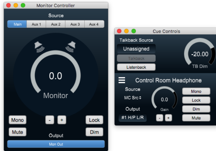
Figure 11.12: Default Monitor Controller and Cue Control windows
