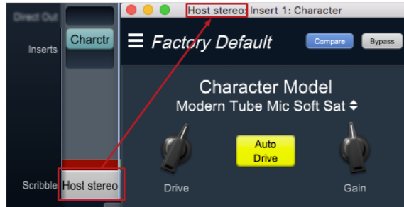
Figure 1.15: Scribble Strip name to Mixer strip Insert header
