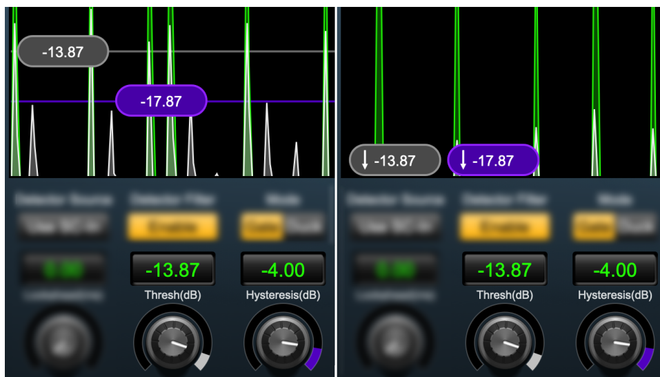
Threshold and Hysteresis controls shown within the display range (left) and below the display range (right)
