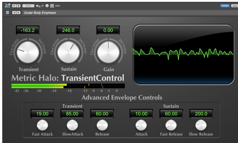
Advanced with Process Metering: Adds Access to the Advanced Envelope Controls
